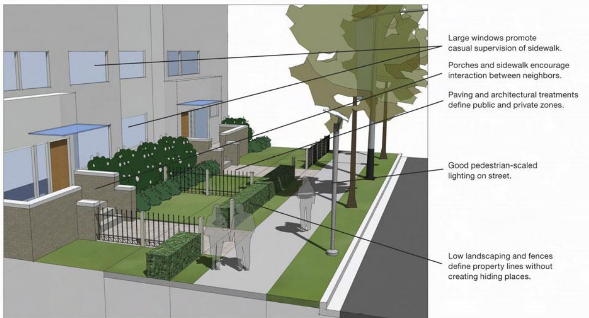
An illustration of some of the example overlay districts’ principles at work.
